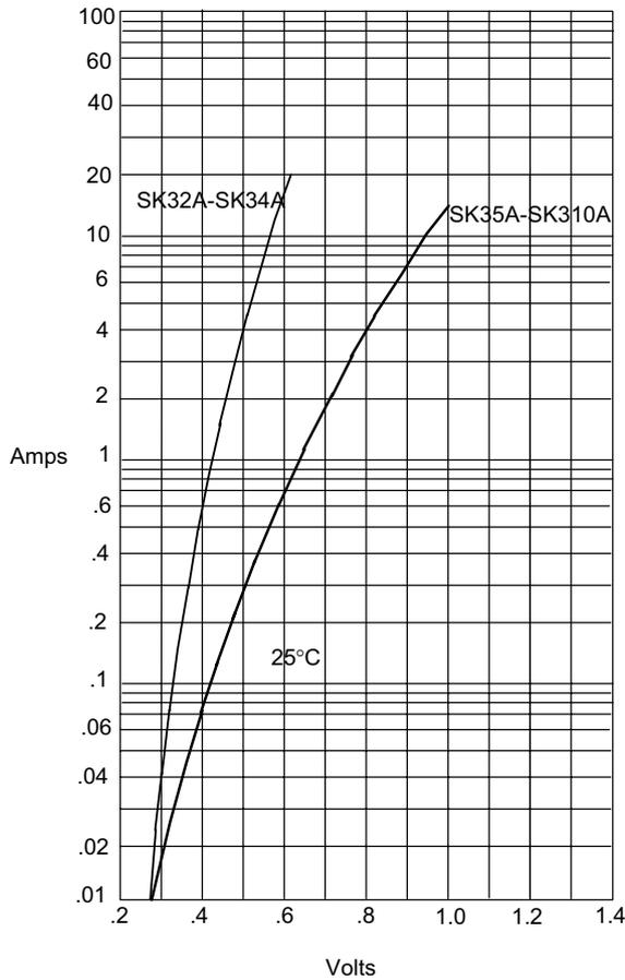
Instantaneous Forward Current - Amperes versus
