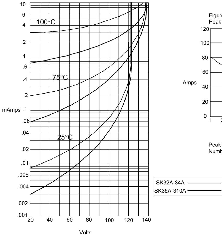
Instantaneous Reverse Leakage Current - MicroAmperes versus
